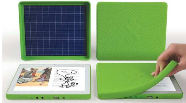
Figure 1: Nell’s solar-powered hardware platform. The tablet design allows for direct interaction.
