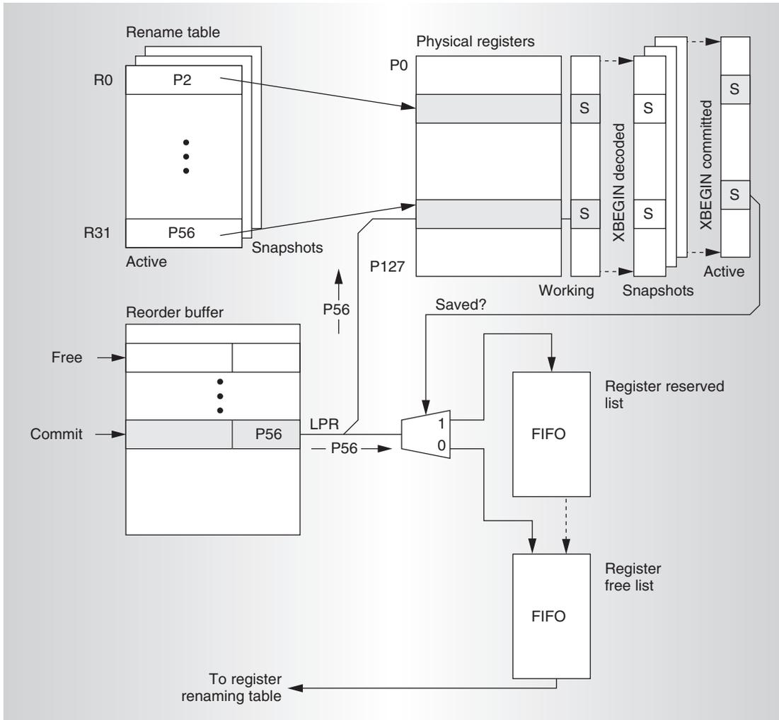
Figure 1. UTM processor modifications. The *S* bit vector tracks active physical registers. For each rename table snapshot, there is an associated *S* bit vector snapshot. The register-reserved list holds the otherwise free physical registers until the transaction commits. The last-physical-register (LPR) field identifies the physical register to free when an instruction graduates (the last physical register referenced by the destination architectural register).
