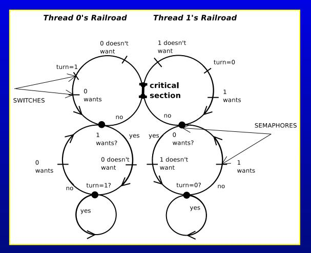
Railroad visualization of Dekker's algorithm for mutual exclusion. The threads "move" in the direction shown by the arrows.
